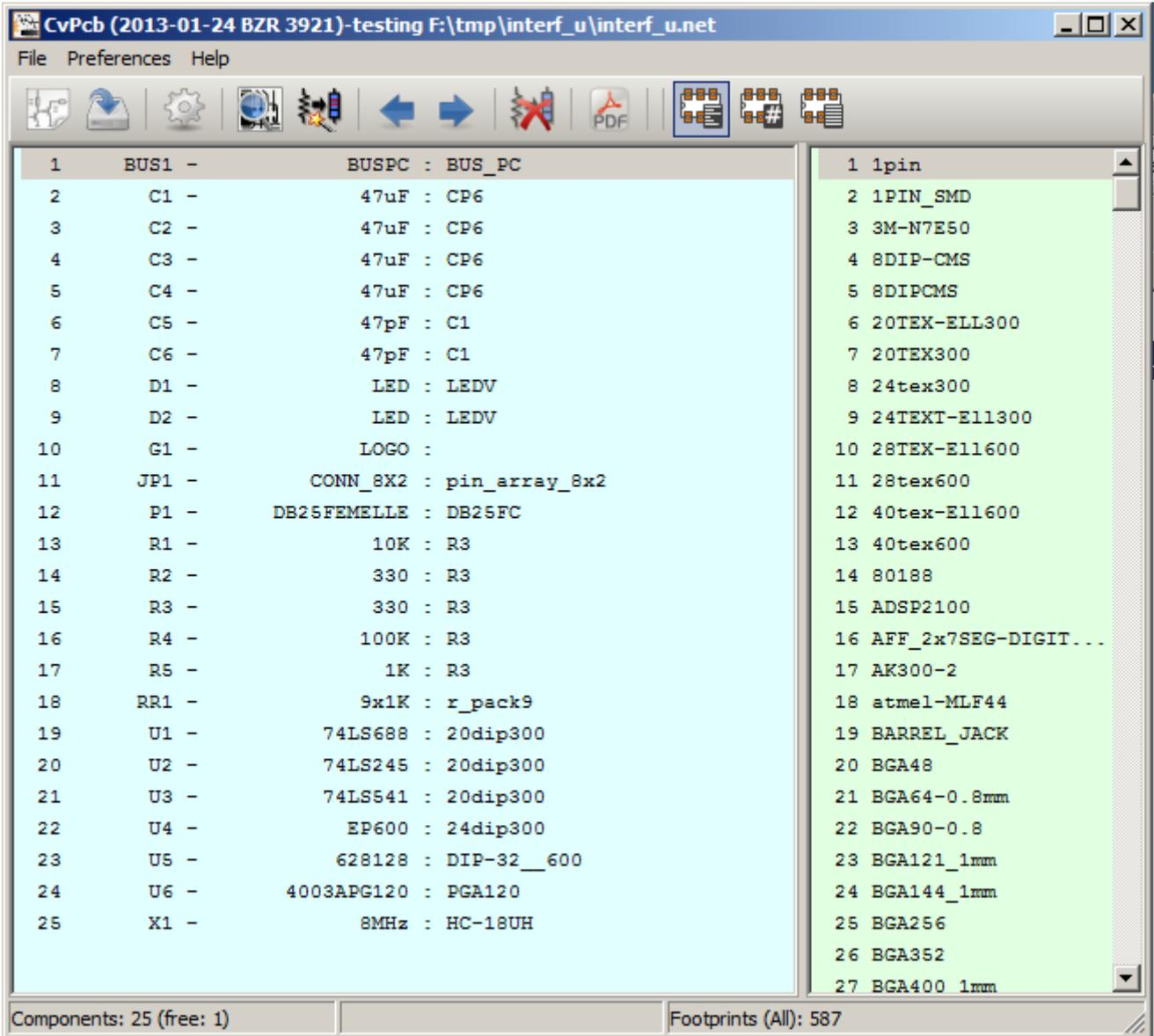
The component window on the left, displays the list of components appearing in the net list file that has been loaded. The footprint window on the right, displays the list of footprints contained in the libraries that have been loaded. The component window will be empty if no file is loaded and the footprint window can be also empty if no footprint libraries are found.
