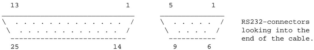
The diagram above represents the Female end of the cable. The male end is the same, but looking from inside the cable.
