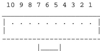
For the serial port DB9F connector, the pin numbers are stamped in the plastic near each pin. In addition, there is a diagram near the end of this chapter.
