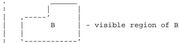
When the program requests a *display context* (DC) for a window it can specify an optional clipping region that further restricts the area where the graphics output can appear. This area is calculated as an intersection of the visible region and a clipping region.
