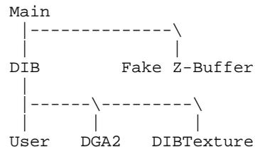
Main provides a very simple base class that does not implement any of the image-related functions. Therefore it does not place any constraints on how the surface data is stored.
