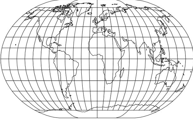
Figure 46: Winkel II,  $\text{+lat}_1=50\text{d}28'$  ( $\cos^{-1}(2/\pi)$ ).
