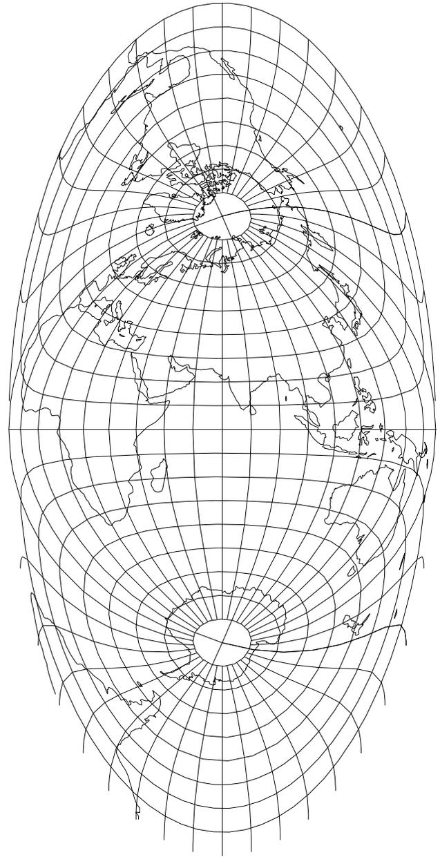
Figure 58: Oblique Mollweide projection proposed by Close, `+proj=ob_tran, +o_proj=moll, +o_lat.p=0, +o_lon.p=90, +lon_0=160. 10°` graticule.
