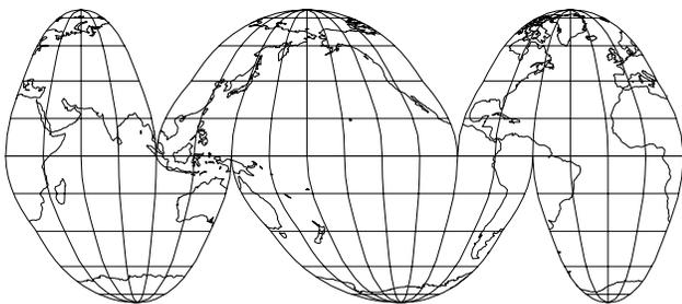
Figure 2: Interrupted Goode Homolosine emphasizing oceanic masses.
